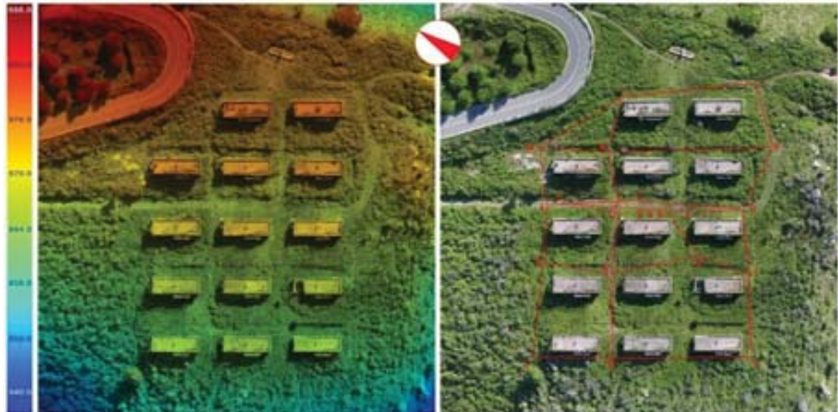
Fig. 3: Orthophoto of the complex and its immediate surroundings, the image highlights the colour range in relation to heights, on the right, orthophoto of the mesh model with topographic polygon and indication of the GCPs used for alignment.
