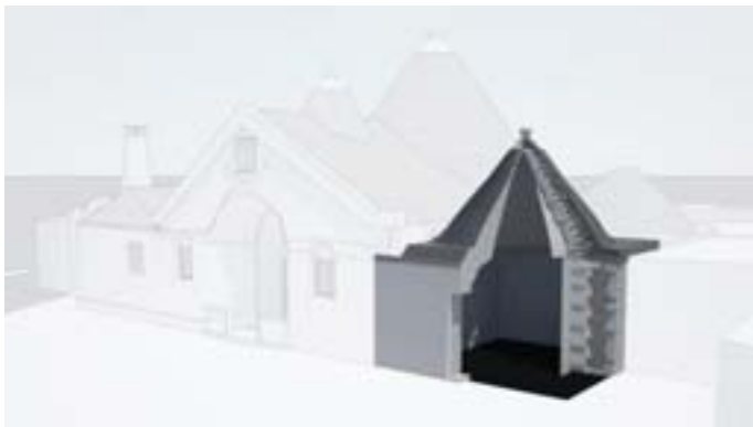
Fig. 1: Alberobello - Bari. Trullo sovrano. Section with masonry and cone structure composition.
