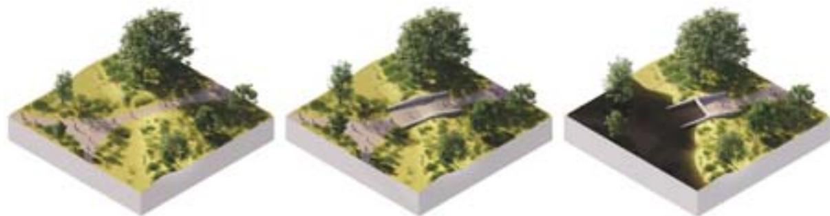
Fig. 6: Phases of construction of the transversal paths that cross the dune defended by retaining walls and anti-water bulkheads and flooding scenario (source: CF MØLLER ARCHITECTS et alii, Bådparken. På kanten af Fjord & By , 2022).
