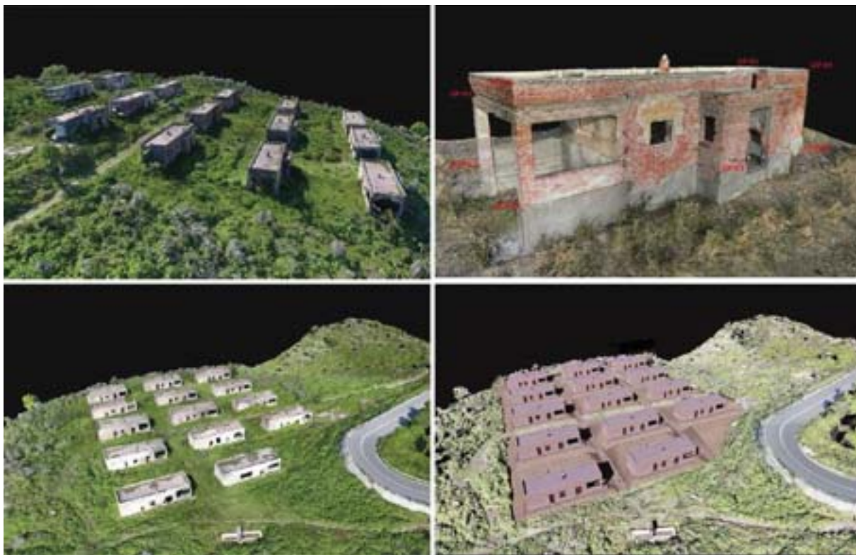
Fig. 7: On the top left side, the textured mesh model of the actual state obtained from SfM reconstruction of the entire Borgo di Pietrapizzuta; on the right, the mesh model of the building sample chosen for the study. On the bottom: left side, image of the mesh model of the village processed from SfM clouds, right side, mesh reconstruction of the buildings and orography of the site area.
