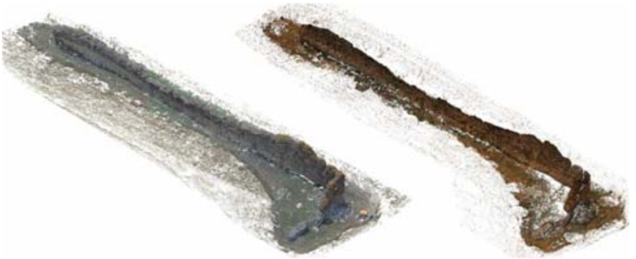
Fig. 7: Point clouds from the photogrammetric and laser scanning survey of the south-west wall section.
