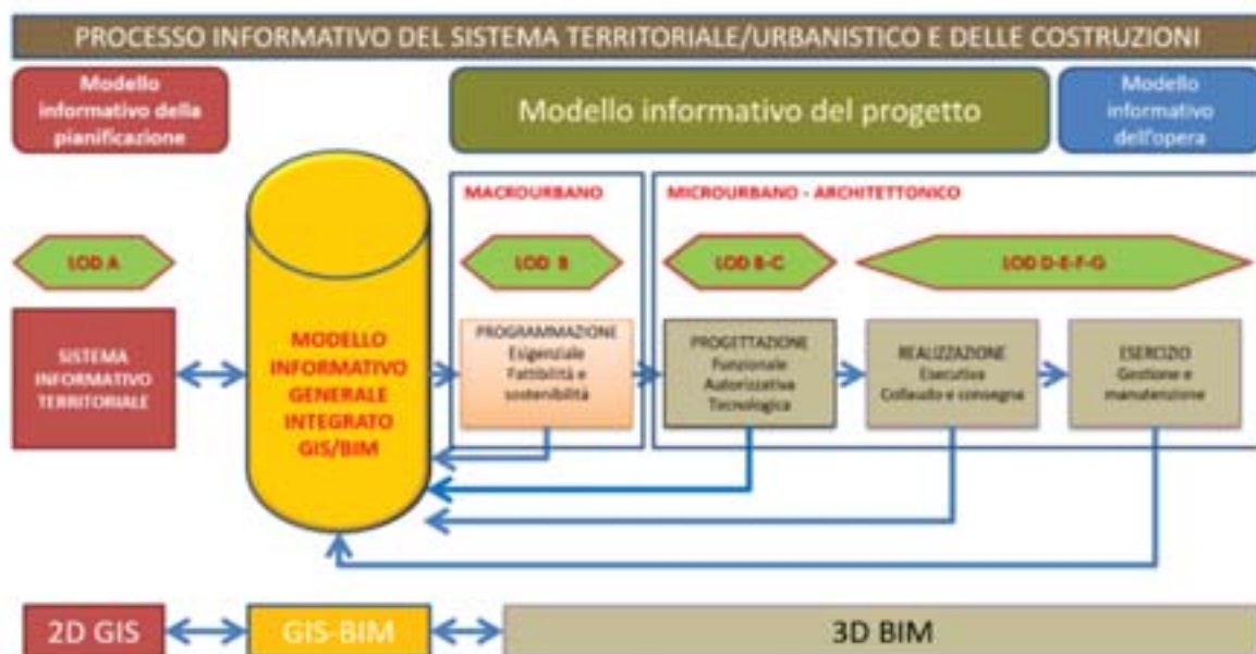
Fig.5: Methodological diagram of the information apparatus structuring through an integrated GIS-HBIM database as the basis for multi-scalar analyses. Source: elaboration by the authors.
