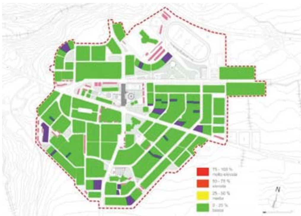
Fig. 2: New Conza della Campania (Av) - Global Urban Seismic Vulnerability Index resulting from the application of the CPD-INEDG method. Violet, is not listed in the legend, public buildings for which vulnerability was not evaluated were highlighted
