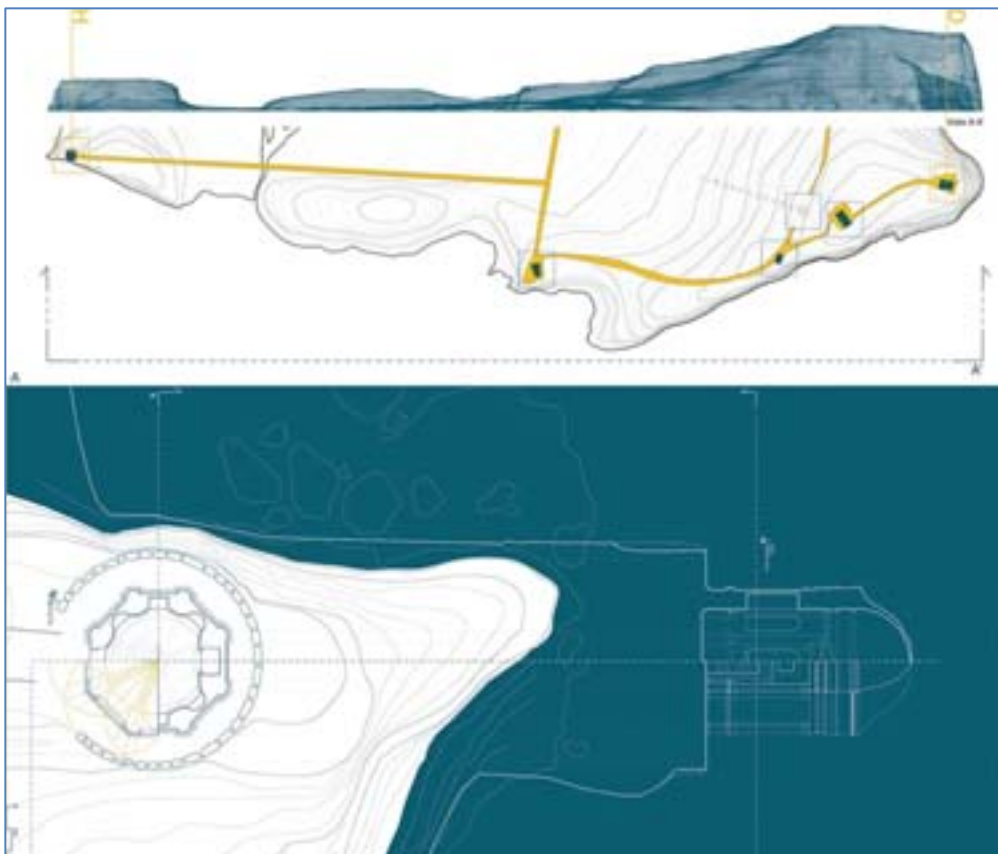
Fig. 6: Surveying the East side of the Bisentina Island, Lake Bolsena, Central Italy. Horizontal and vertical section of the oratory of Santa Caterina. General plan and view from the AA section plan of the terrain model. Highlighted in yellow color, the historical paths that connect the Oratories located on the peaks, (from left to right): oratory of Santa Caterina on the 'Rocchina'; oratory of the Crocefissione on the 'Monte Calvario'; oratory of San Gregorio near the Well of the Malta Dantesca (dashed); oratory of the Trasfigurazione on the 'Monte Tabor'; oratory of the Orazione all'Orto on the Monte Uliveto. [Drawing by Authors].
