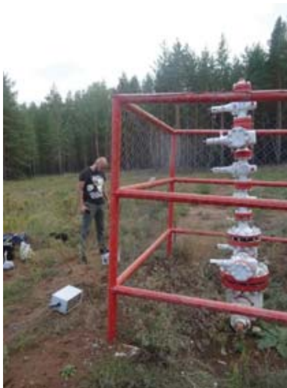
Fig. 2: Measurements of gas emissions near the well No 107 of Mogutovskoye oil field of Orenburd region.
