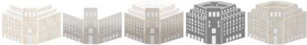
Fig. 4: The sequence of the methodology includes: a photogrammetric campaign, a survey using a lidar scanner, the union of the two point clouds to obtain more accurate data, the creation of the energy model, the settings of the casing materials and systems.
