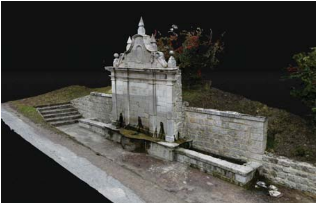
Fig. 10: Image of the polygonal mesh of the fountain with textures.
