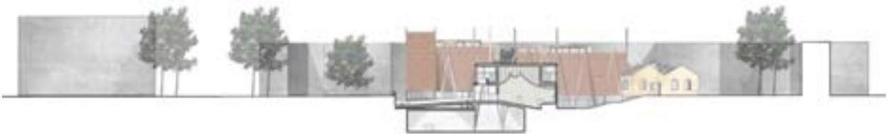
Fig. 10: Section of the building. It is possible to see the inside of the auditorium and in the background the facade with the brick sunscreens.
