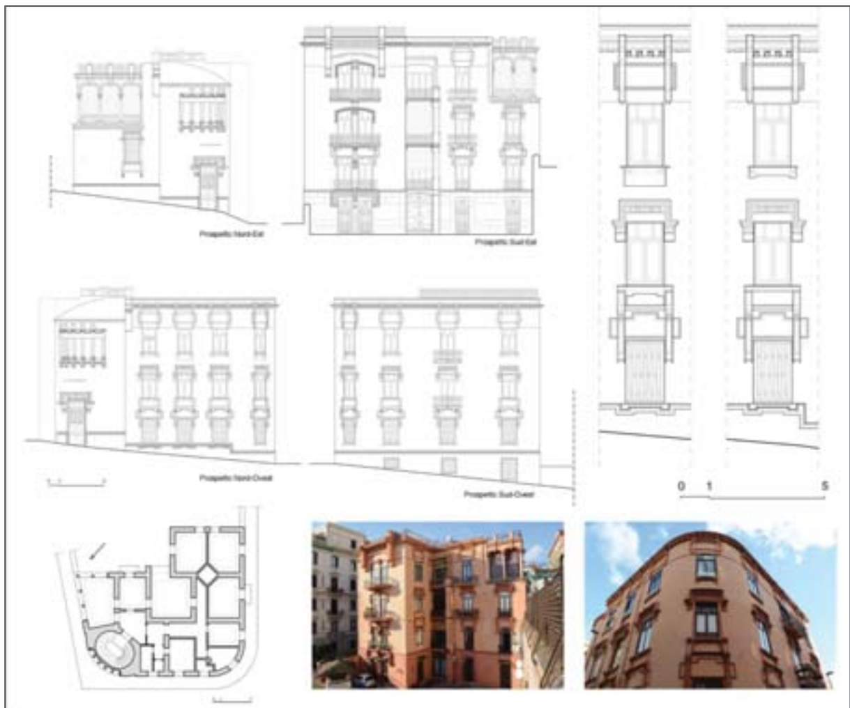
Fig. 4: Villa Loreley. Image of the building seen from via Palizzi with the loggia. Graphic representation in orthogonal projection of the façades on the bend of via Gioacchino Toma and on the private garden. Floor plan of the typical level. Architectural details of the façade.
