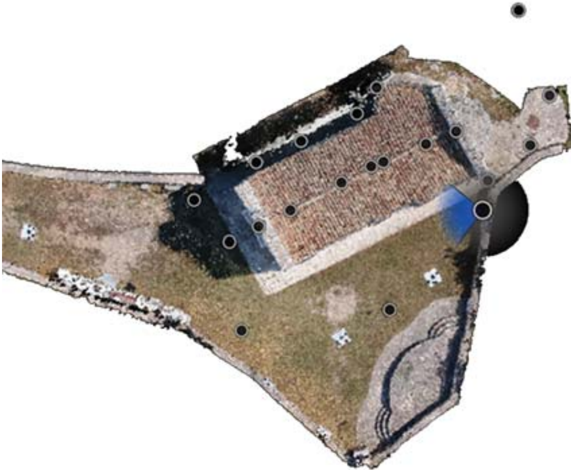
Fig. 4: Planimetry points station LIDAR
