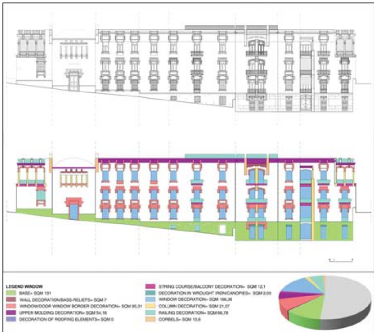
Fig. 7: Villa Loreley. Comparative analysis between the development of the facade on via Gioacchino Toma with architectural details and synthesis scheme of the decorated surfaces. Histogram representing the incidence of the decoration in relation to the area represented.
