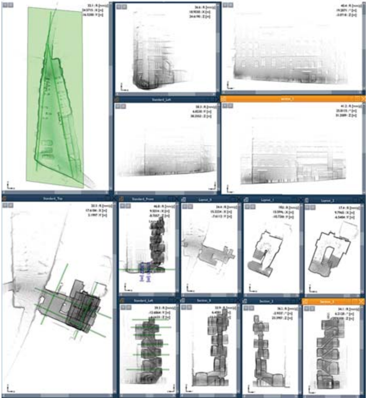
Fig. 5: Top left: Coloured dense point cloud performed with the GEO Slam HORIZON Portable Laser of the portion of the historical centre investigated; followed by graphic elaborations of synthesis of the monochrome dense cloud performed with the GEO Slam ZEB GO Portable Laser of Piazza Pinelli and the elevations facing it. Finally, elaborations of plans and sections obtained from the dense cloud of the atrium and the stairwell.
