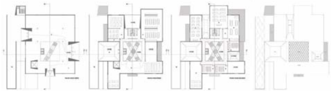
Fig. 3: Succession of plans, from the ground floor to the roof plan. The central atrium with the skylight characterized by the same design as the stained-glass windows of the Basilica and the other impluvia that cover the terraces are visible.
