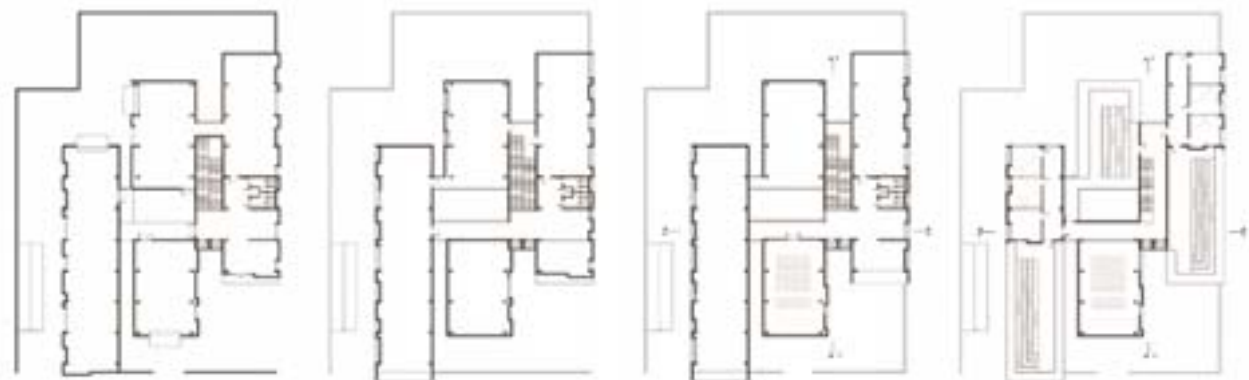
Fig. 2: Succession of plans, from the ground floor to the top floor. Note the three parts joined by the connective spaces.
