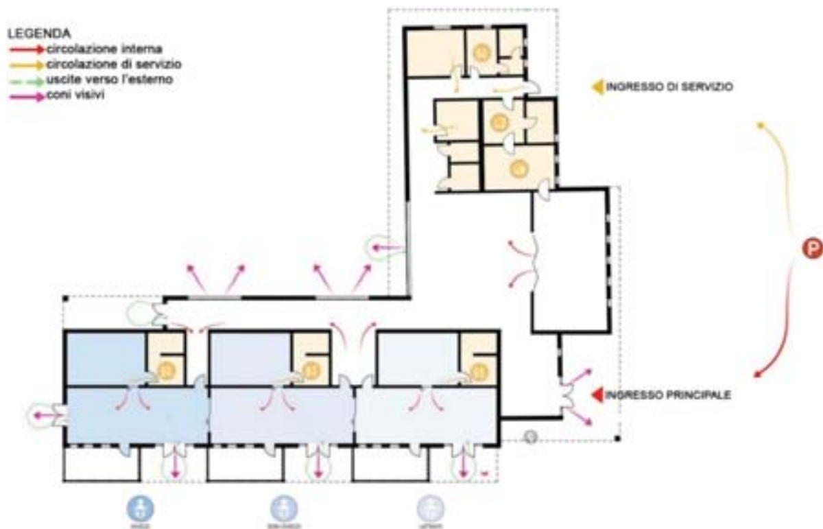
Fig. 6: Project for the construction of a nursery school in the Municipality of Baronissi: plan with indication of internal flows and relations with the outside.
