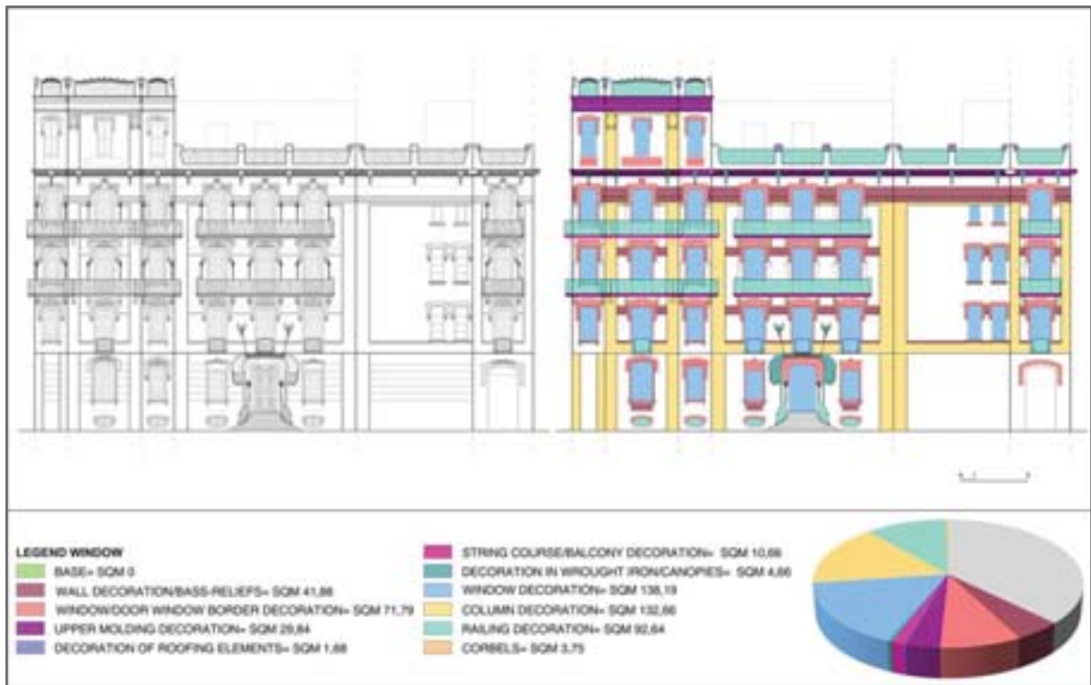
Fig. 8: Villa Pappone. Comparative analysis between the development of the facade on via Salita del Casale with architectural details and synthesis scheme of the decorated surfaces. Histogram representing the incidence of the decoration in relation to the area represented.
