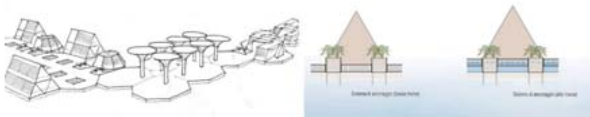
Fig. 8: Left: sketch of the node connecting the two settlements. Right: scheme of anchoring and floating of the platform in the different phases of the tide. Graphic elaboration by S. Puglisi and A. Siligato.
