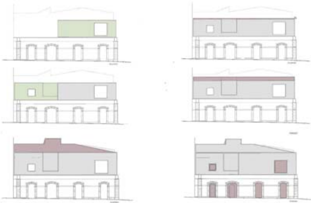
Fig. 6: Assembly phases of 3D printed elements on-site and off-site
