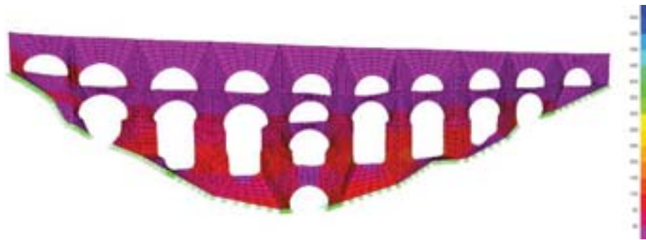
Figure 14. Bending stresses for the 5-ELU combination.
