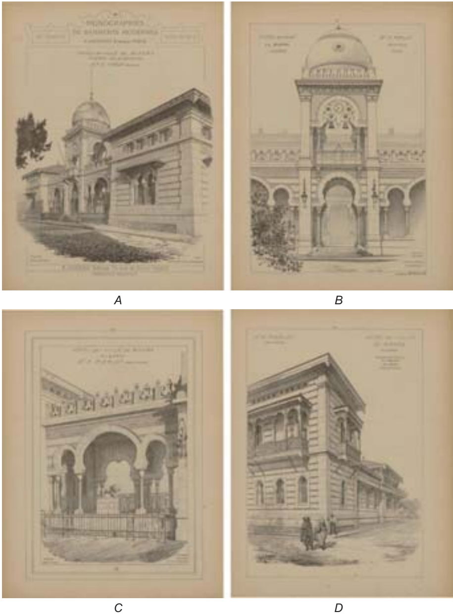
Figure 16. Graphic drawings showing details of the distinctive elements of the city hall of Biskra: A) main façade; B) details of the campanile; C) covered vestibule and lion statue; D) the wooden balconies [56].
