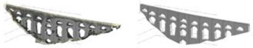
Figure 8. Model created in Autodesk Revit 2022 overlaid with the point cloud.
