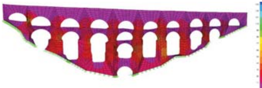
Figure 15. Shear stresses ( V_{max} ) for the 5-ELU combination.
