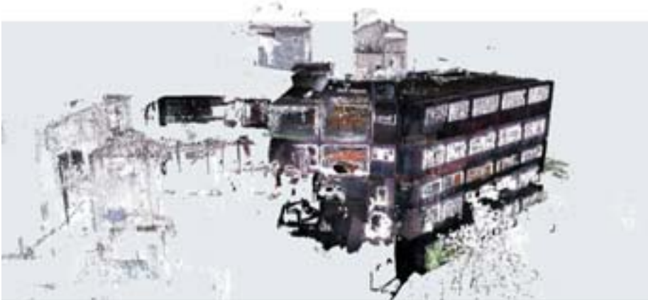
Figure 9. Final point cloud of the paper mill (Source: Antonio Landa).
